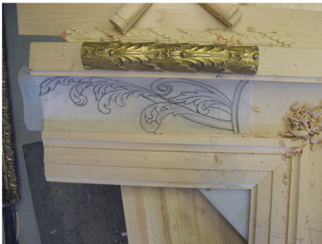
41. Five-foot mold for the ornament on the crossmembers of the frame {fix}
